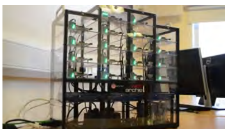
Figure 1: Wee-Archie: a small 64 core cluster made out of 18 Raspberry Pis.
