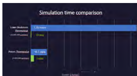
Figure 3: On the top LA, on the bottom Peters: CPU time is in blue, GPU time is in green.
